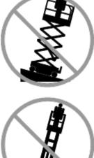
Do not raise the platform unless the machine is on a firm. level surface.
