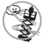
Do not operate the machine in strong or gusty winds. Do not increase the surface area of the platform or the load. Increasing the area exposed to the wind will decrease machine stability. Do not modify or alter a mobile elevating work platform without prior written permission from the manufacturer. Mounting attachments for holding tools or other materials onto the platform, toeboards, or guard rail system can increase the weight in the platform and the surface area of the platform or the load.
